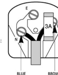
A fused plug must be fitted with a 3A fuse approved by ASTA or BSI to BS 1362 and fuse covers must always be securely replaced.
